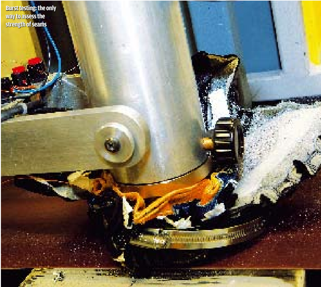
Preparing the gloves for the burst test
